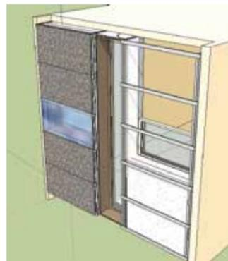
The main components of future experimental facades: construction, insulation and external covering
